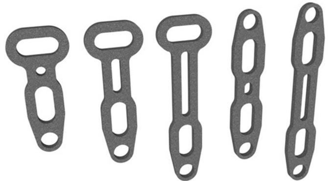
Fig. 3. As a result of this study, the company changed the design. The arms have been broadened by 0.35 mm to increase the S–N fatigue curve. The circle of the hole for the third screw has been made complete.
